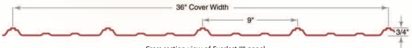
Cross section view of Everlast II® panel
